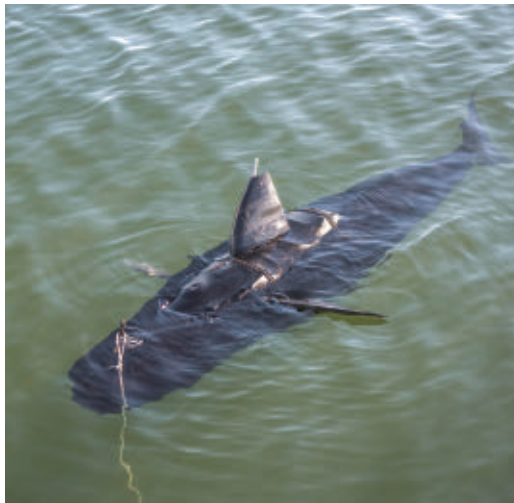
The GhostSwimmer UUV from Boston Engineering is designed to mimic the behavior and movement of a fish to preserve stealth for military missions like surveillance, mine countermeasures, port security, and similar defense and homeland security applications.
